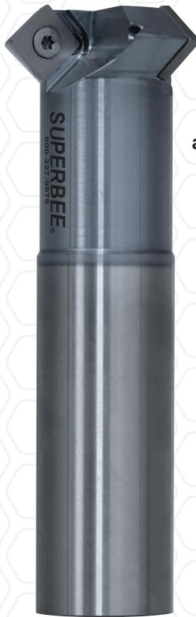
Ideal for cutting a 45° on the top or bottom of a part, utilizing a square 4 cornered insert, and stocked with 5 different radii. The positive geometry allows for more aggressive cutting action, while the proprietary pocket design provides unmatched repeatability and reduced runout.
